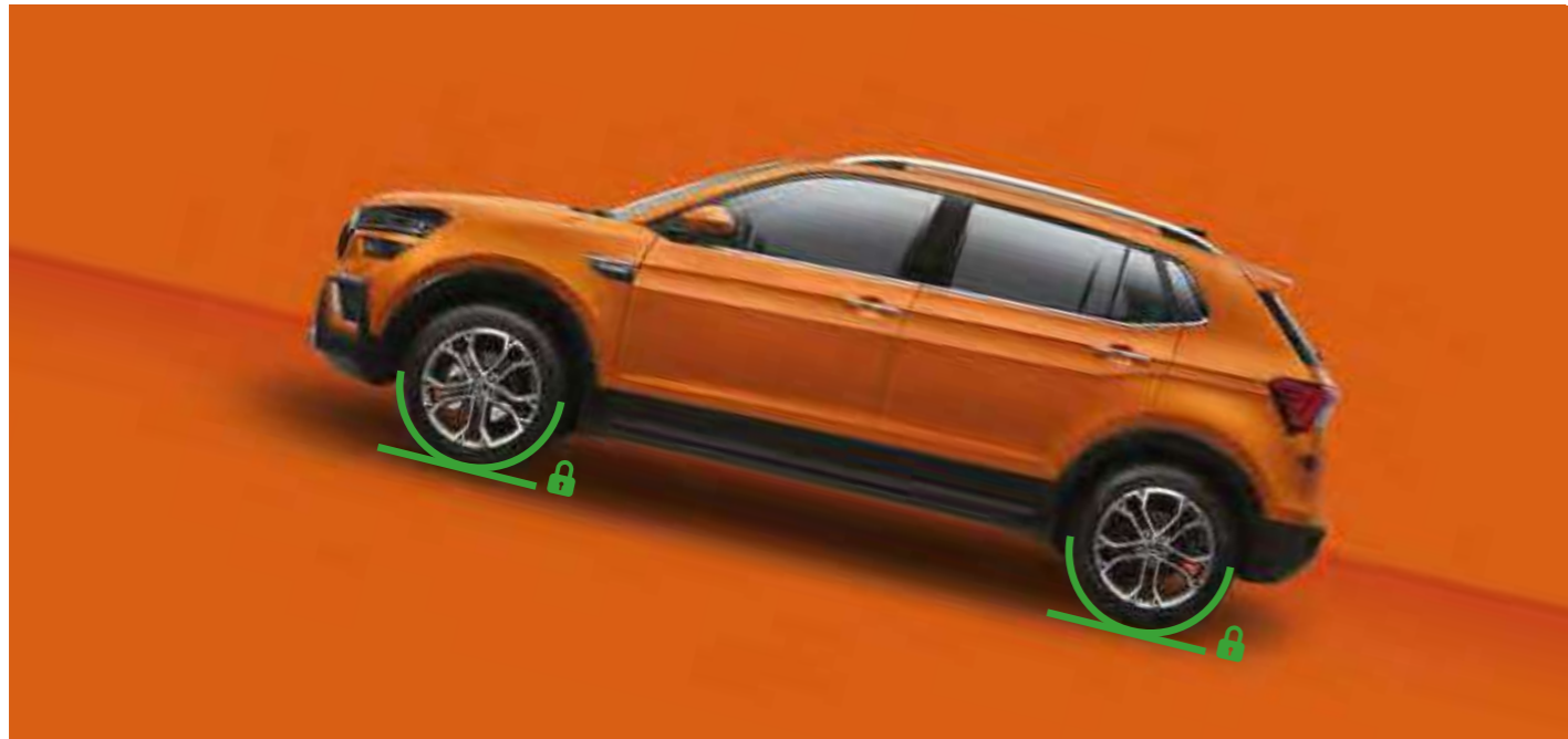
Hill Hold Control HHC allows a safe start uphill without using the parking brake.
