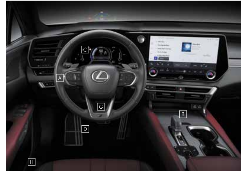
F SPORT Performance/ A_Dimpled leather steering wheel with paddle shifters / B_Dimpled leather shift knob / C_TFT meter / D_Aluminum sport pedals and footrest / E_Real aluminum ornamentation / F_Leather sport seats
