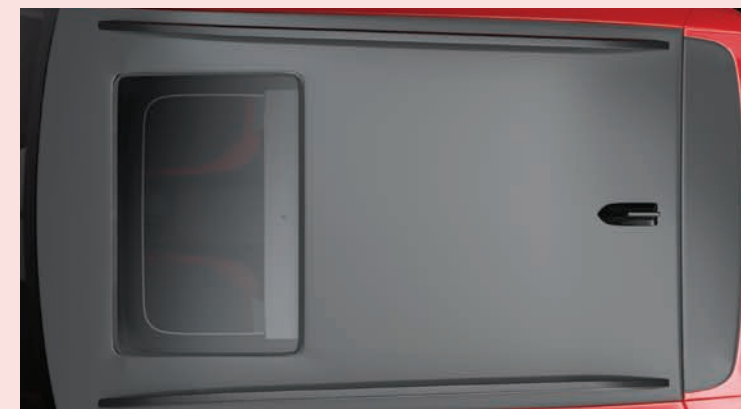
Carbon Steel Painted Roof
